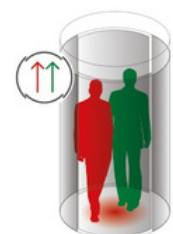
PIGGYBACKING: DETECTION VIA WEIGHT SYSTEM AND STEREOVISION
