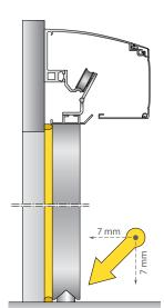
Door in lowered and closed position, the wing offers a tight all-round seal.
