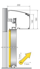
Gilgen SLX-D automatic hermetic door with drip-off covering, running carriage shown in open door position.
